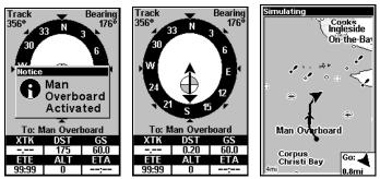
Navigating to Man Overboard: Man Overboard activated (left), Navigation Page (center), and Map Page (right). The victim is astern of the vessel. The GPS shows which direction to steer to for the rescue.
